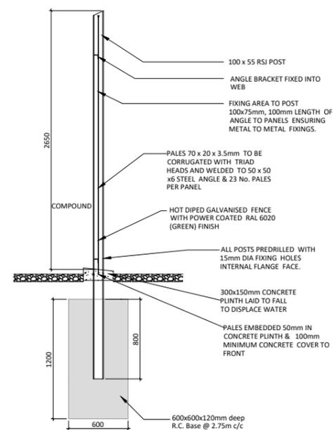
**Typical Palisade Fencing Details - Section**
